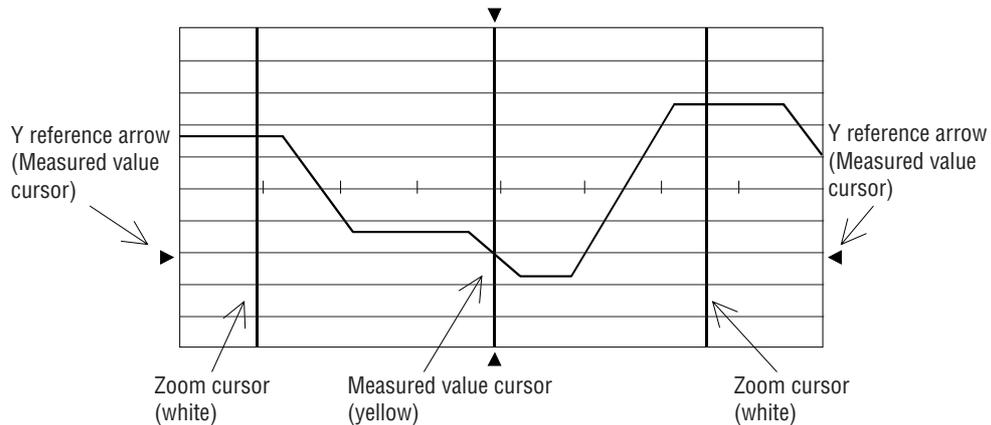
**Figure 31:** The MD\_SCOPE plot area
