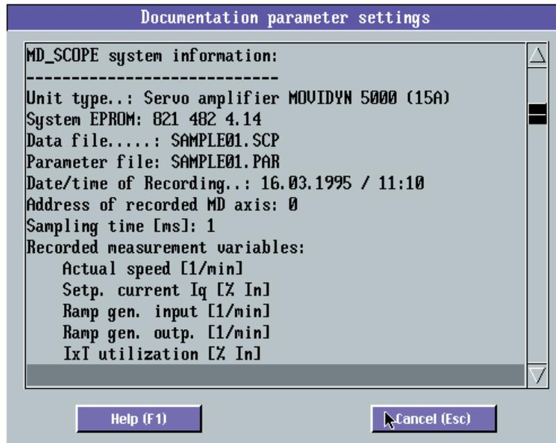
**Figure 11:** Documentation of MD\_SCOPE and MOVIDYN® parameters
