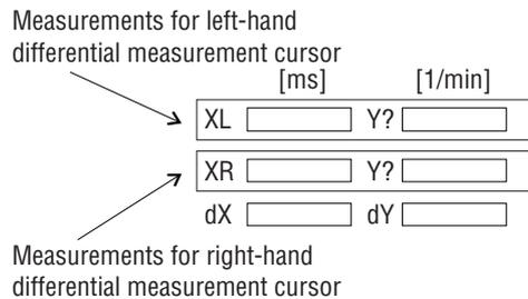
Figure 3: Numerical display of differential measurements
