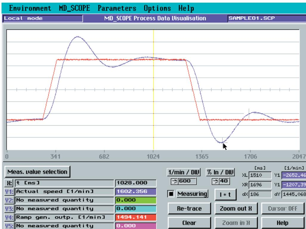
Figure 4: Window with activated differential measurement
