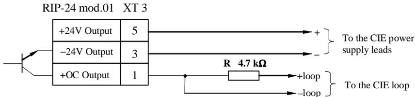
R is the Loop End-Of-Line Terminator provided with the CIE; it is to be installed within the RIP-24 enclosure
