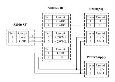
Figure 1: S2000-ST Detector Wiring Diagram
