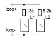
L1 – tamper lead L2 – detector lead
