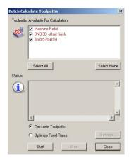
Te form appears with all of the **toolpaths** listed. By default all of the toolpaths are ticked, ready to be included in the **Batch Calculate** process.
