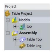
Note: A project is associated with a (\*.3dp) file extension. When a project is opened, all associated ArtCAM models and Assemblies are opened with it.
