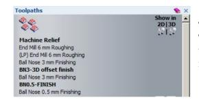
The Unprocessed **toolpaths** are displayed in thr Toolpaths Tab. In addition, there are no '**display toolpath**' tick boxes below '**Show in 2D/3D**' indicating that they have not yet been calculated.
